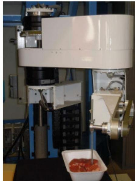
Fig. 2. *In vitro* relaxation test using D2M2 robot
